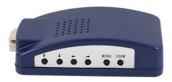
LKV2000 converts PC VGA to composite (Yellow RCA) and/or S-video TV display signal. It is with a VGA pass through so that you can keep your computer monitor connected while sending a signal to the TV. All outputs are loopthrough, display simultaneously. It is with fine tuning control to adjust the picture to your preference. It draws power from an available USB port using a supplied USB power cable. No external power supply is needed.
